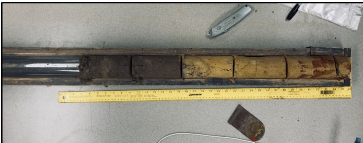
Figure 2.12. This is an intact extracted soil core sample that was segmented and later separated for soil texture analysis.
