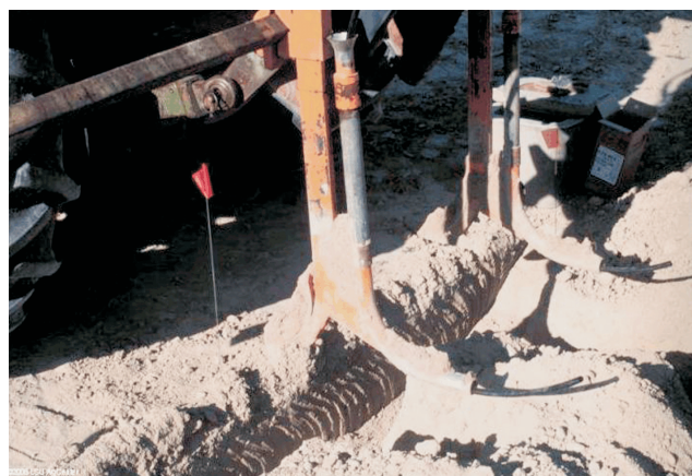
Figure 2. View of a drain plow used to install subsurface drip irrigation tubing.
