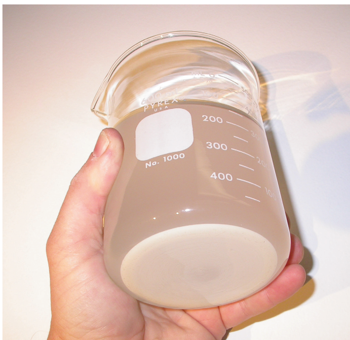
Figure 14. Several liquid spray formulations (wettable powders, suspension concentrates, and micocapsules) form true suspensions, and will settle out of water when given sufficient time. In these photographs, a suspension concentrate was diluted in water at 4:00 p.m. (top photograph). The following morning, the solid, particulate matter had settled to the bottom of the glass beaker (bottom photograph), and required agitation to re-suspend the product.
