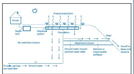
The figure to the left demonstrates how effluent from on-site wastewater treatment systems may reach ground water or surface water. This figure demonstrates the importance of proper siting of on-site wastewater systems
