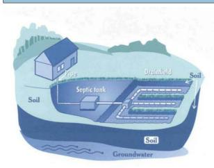
On-site wastewater treatment systems provide treatment and ultimate dispersal of wastewater from homes and small businesses. They usually consist of a septic tank, a drainfield, and the underlying soil. When properly designed, installed, and maintained on suitable soils, on-site systems are an environmentally benign method to manage household wastewater. With proper care and maintenance, an on-site system should function properly for at least 20 years.
