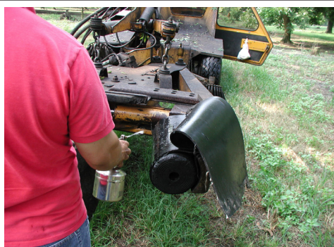
Figure 7. Application of silicon get between the flap and pad of a pecan shaker to prevent bark damage to pecan trees.
