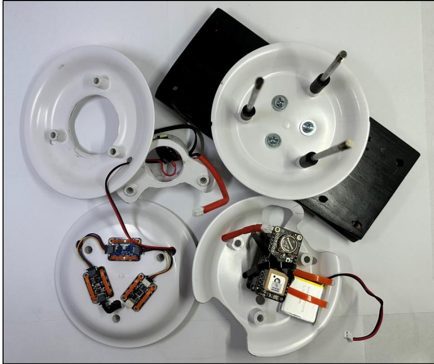
Figure 22. Fully disassembled DSU revealing placement of the microcontroller stack and battery, as well as how it is attached to the wood plank.
