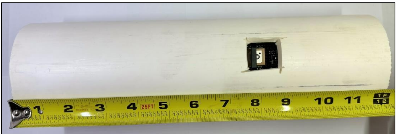
Figure 15. Assembled VSU. The GPS receiver is visible through the top.
