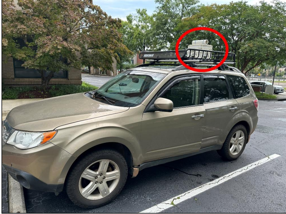
Figure 18. Collection vehicle equipped with the VSU (red circle).
