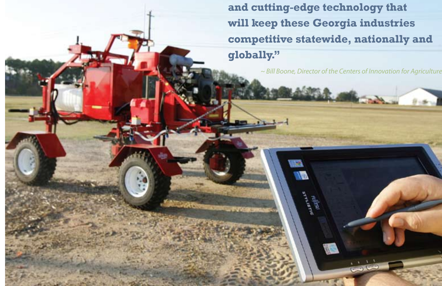
Developed on the Tifton campus, the sipping tractor is operated by remote control and uses the smallest amount of energy required.
