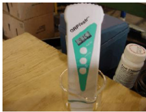
Figure 42. Using ORP meter to measure chlorine activity in wash water.
