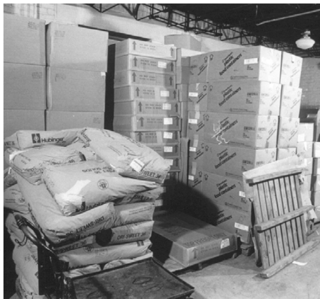
Figure 2. Dry Ingredient Storage Area. Keep materials, ingredients and supplies off the floor and in closed containers. Repair torn bags.
