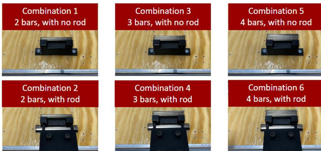
Figure 4.2. The orientations of the tested bar and rod magnets.
