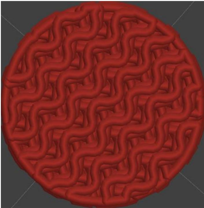
Figure 2.11: Top view of a 50% gyroid infill model in the PrusaSlicer software showing pore structure.
