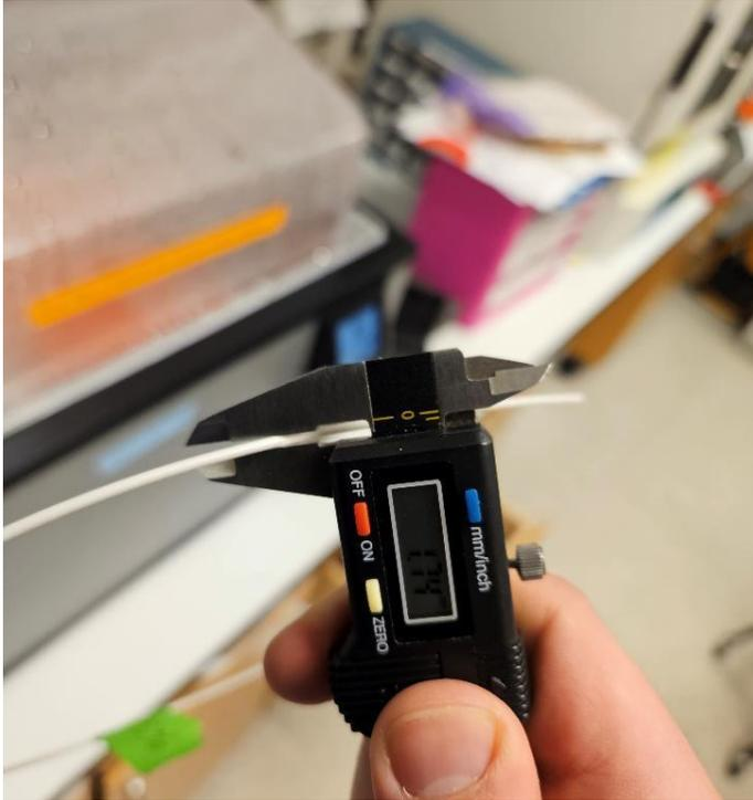
Figure 2.6: An extruded filament being measured; units are in centimeters.
