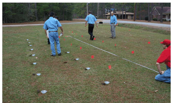
Figure 5. Installing catch-cups for a uniformity analysis at one of the audit sites.
