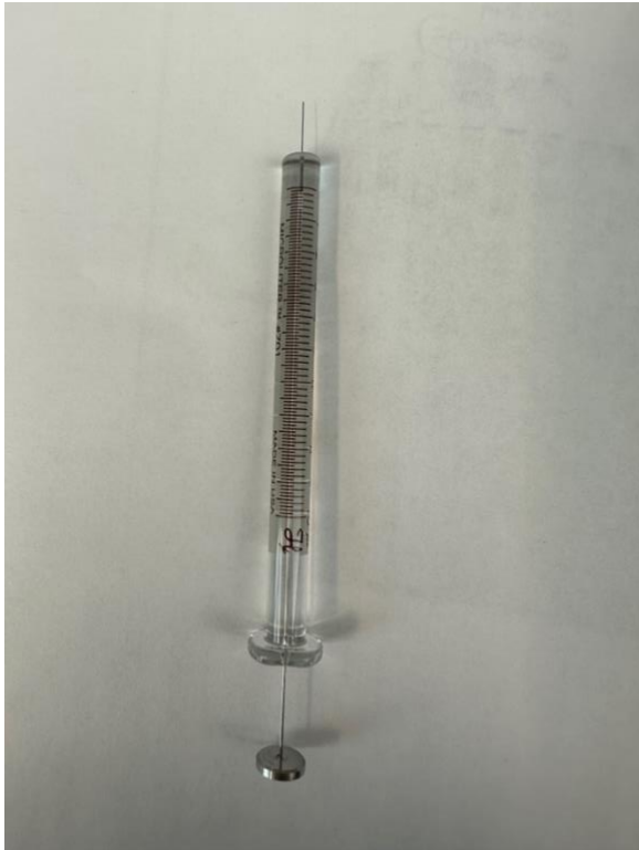
Figure C.1. Custom-made Hamilton syringe and its tip
