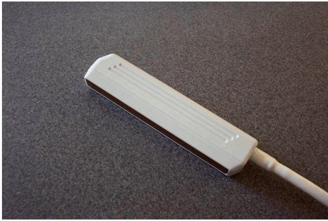
Figure 1. An ultrasound transducer houses tiny crystals that emit and catch the sound waves.
