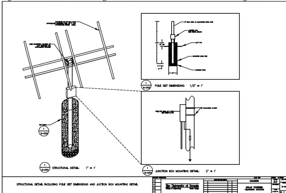
Figure 3: Pole Installation Dimensions and Direct Burial Detail
