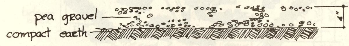
Loose Aggregate Paving scale 1"=10"
