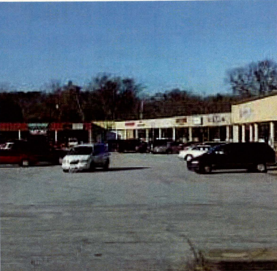
A lack of organization within the parking lot (particularly lane lines and a lack of well-marked parking bays) causes confusion and many fender benders.
