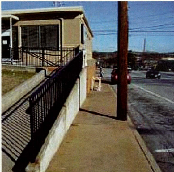
Congested sidewalks create challenges for pedestrian use. A 5' sidewalk with a left side bordering 9' retaining wall and a right side parallel parking space creates a virtual alley.
