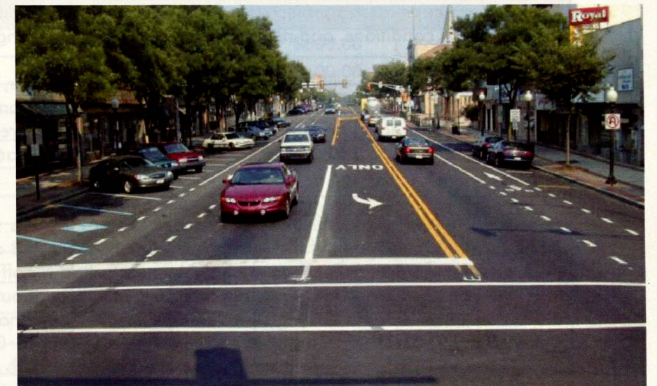
Same street shown after road diet. Using the same roadway width, this street has been transformed to have angled parking, two bicycle lanes, two travel lanes, and a center two-way turn lane, while existing parallel parking has been kept.
