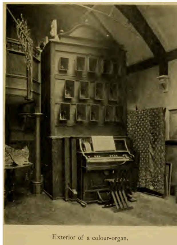
Figure 4 – An example of a color organ. Lights are emitted through the boxes, which have different colored gels in front of a bulb to filter the color of the light. A keyboard-like mechanism is used to control the lighting. 30
