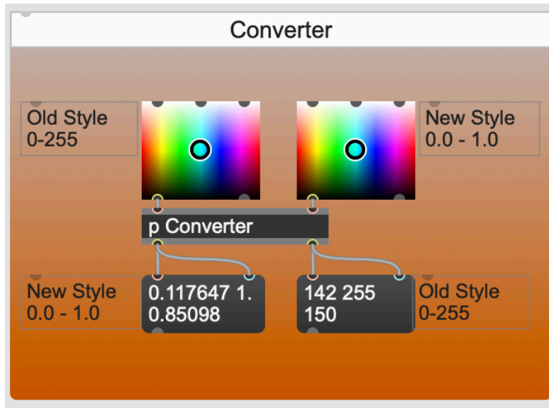
Figure 43 – [p Converter] converts between old (0-255) and new (0.-1.0) style color values.
