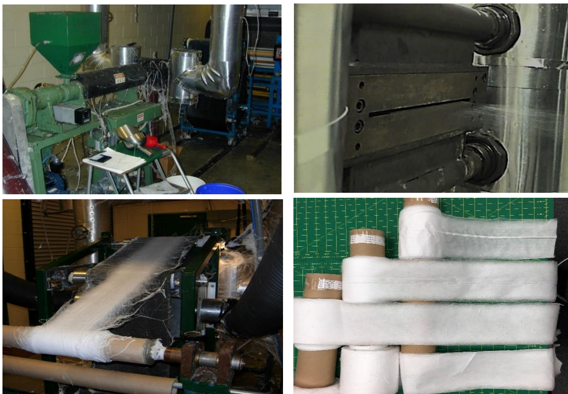
Figure 3.1. Meltblown Pilot Line Equipment and Produced Webs
