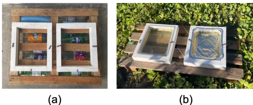
Figure 3.2 Floating minipans: (a) white wooden frames on raft and (b) wooden raft with minipans consisting of a plastic pan (left) and aluminum pan (right).
