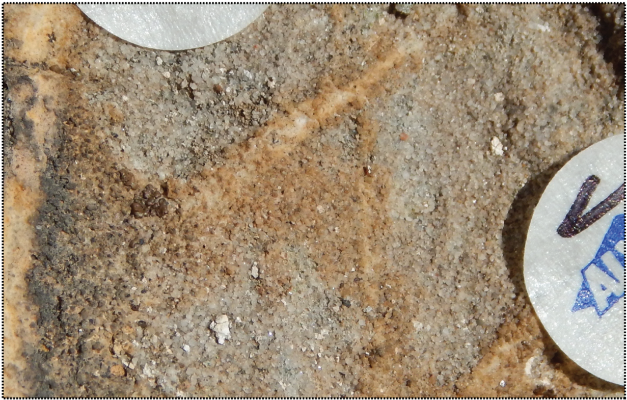
Figure 6. Deformation bands hosted in the Lytle Sandstone in the Mixing Bowl field area. Notice the change in grain size between the deformation bands and the porous Lytle Sandstone.
