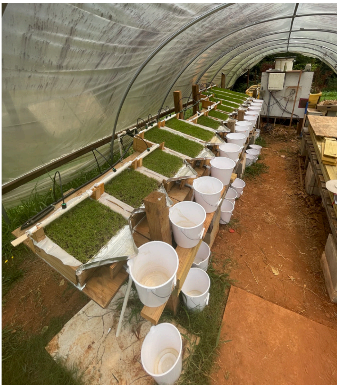
Figure 2.3. All buffer zone plots on bench in greenhouse. Runoff collection in topmost buckets, and subsurface drainage collected in bottommost buckets.
