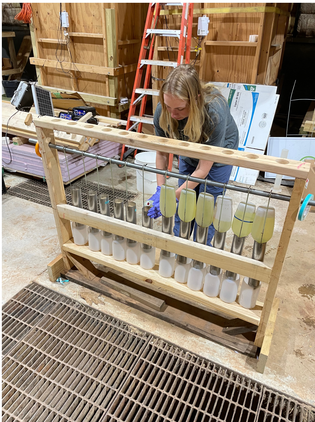
Figure 3.4. Bailey Williams flushing yellow dyed PFAS mixture through stainless steel columns with effluent collection bottles below.
