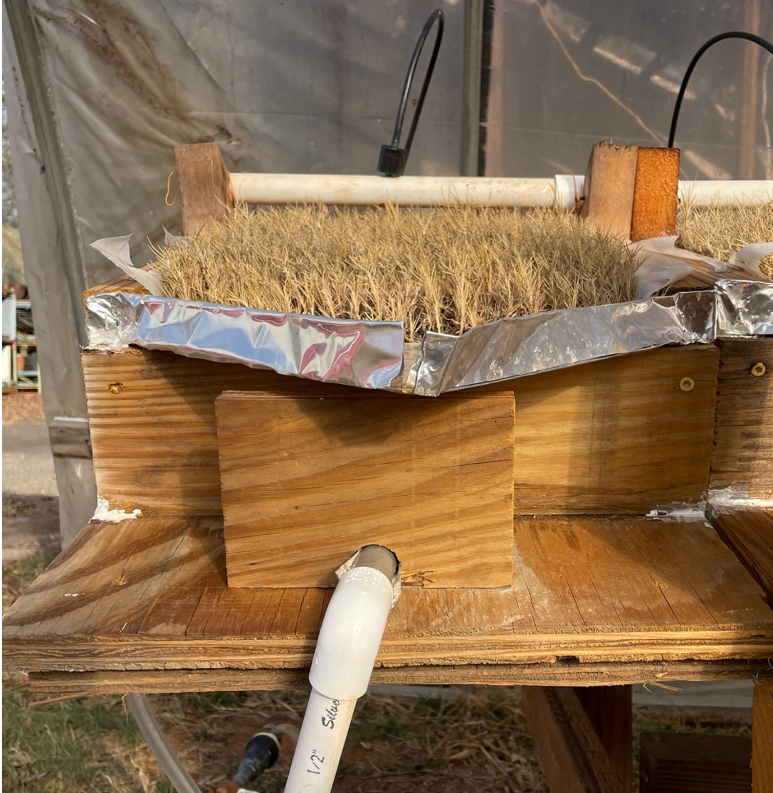
Figure 2.1. Front view of buffer zone plot with drip irrigation pipe located above the plot and subsurface drainage pipe diverting water down and out of the plot. Aluminum flume was attached to plots to divert runoff to a collection bucket.
