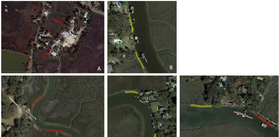
Figure 2: The area of influence of each structure was determined by surveying the streambanks 50 meters adjacent to each structure. Stream banks adjacent to a living shoreline are indicated in red, and those adjacent to a bulkhead are indicated in yellow. Note, a bulkhead and a living shoreline are installed directly adjacent to one another at Little St. Simons, meaning only one side of each structure was surveyed at that site. While this “combination” site is unusual to the present study, it represents a situation that would likely be encountered by a landowner and was included for this reason. Upstream and downstream locations are marked “U” and “D” respectively.
