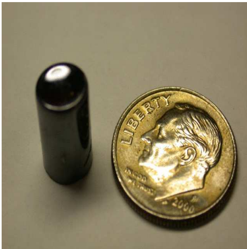
Figure 3.2: \text{As}_2\text{S}_3:\text{Er}^{3+} sample shown with a dime for size comparison.
