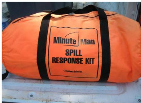
**Figure 2.** Spill kit used to control chemical spills.
