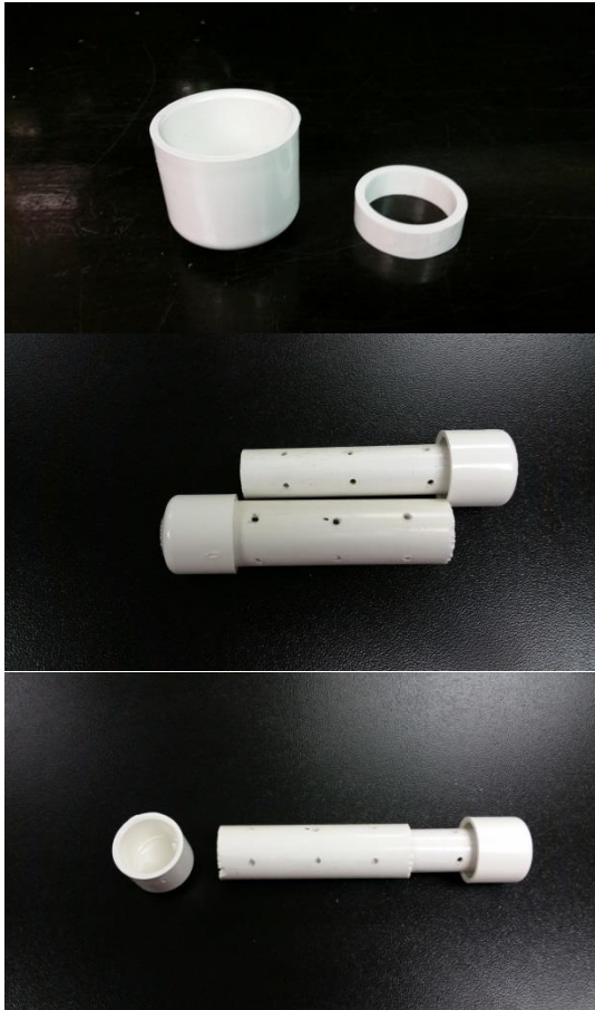
Figure 3.2: Reusable top loading bait trap showing the inner and outer sleeves which can be rotated into an open and
