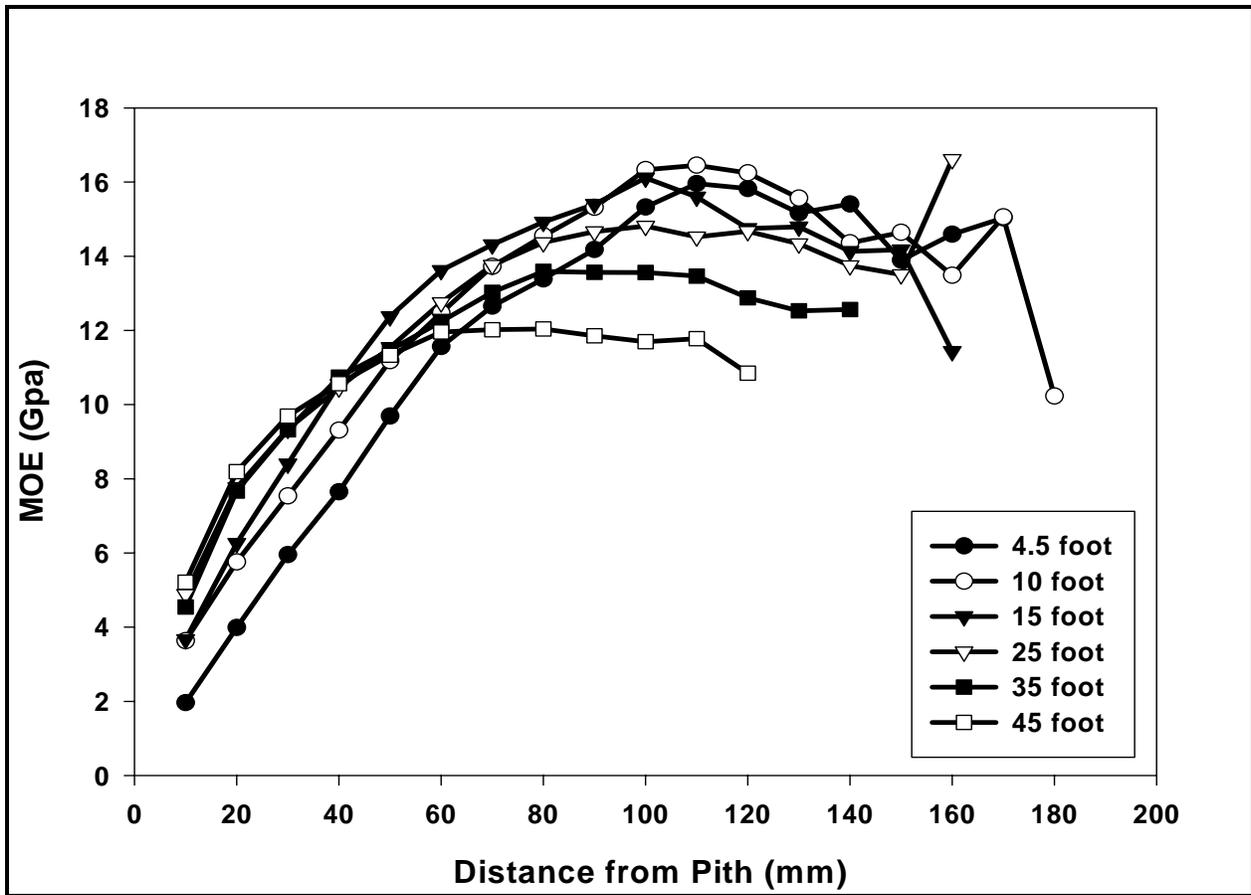
Figure 4.2: Plot of average modulus of elasticity (MOE) versus radial distance by disk height.
