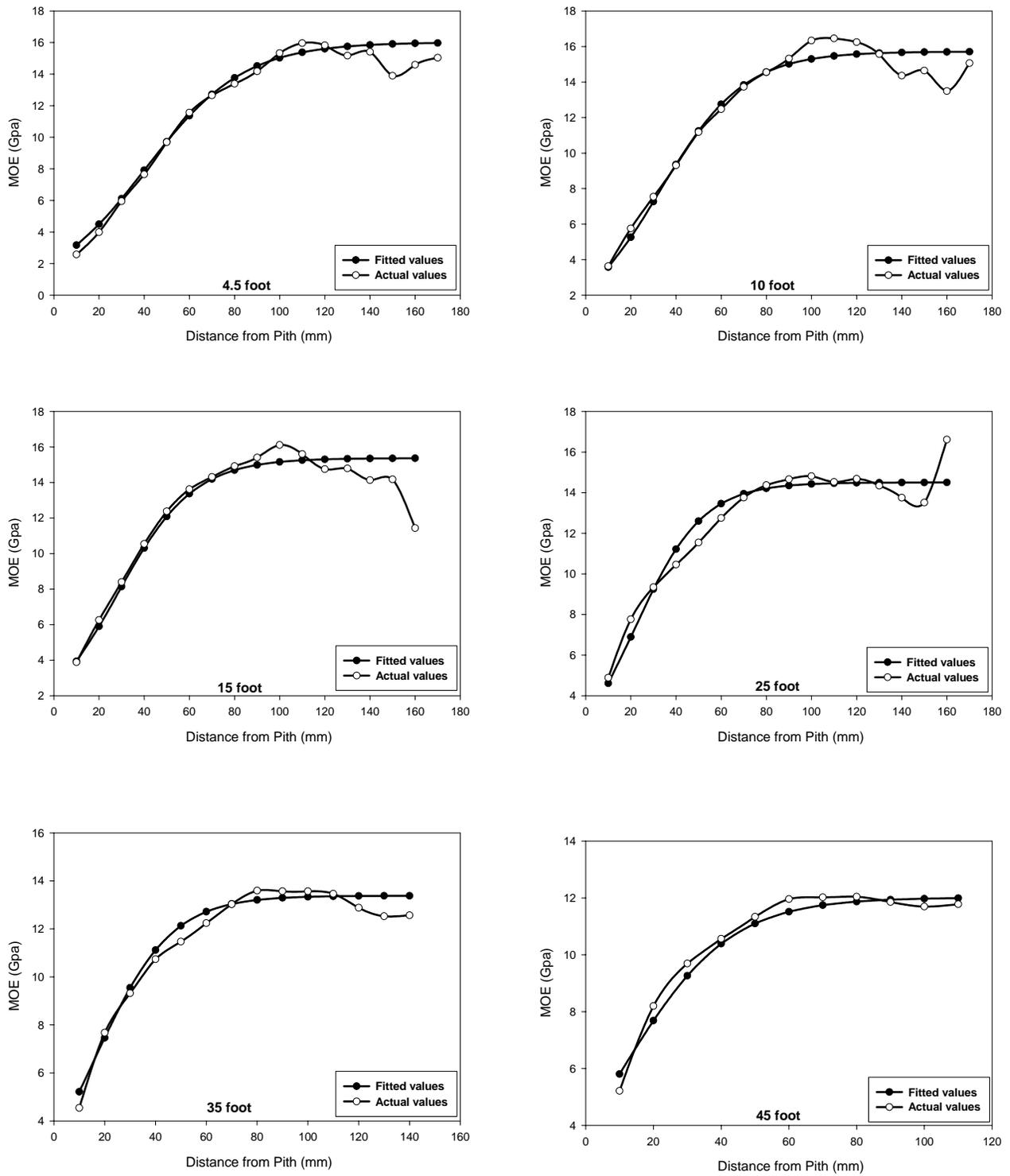
Figure 4.6: Plots of mean actual values versus mean fitted values for the nonlinear modulus of elasticity (MOE) model by height levels.
