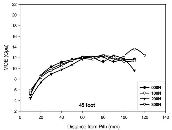
Figure 4.3: Plots of modulus of elasticity (MOE) versus radial distance by treatment at different height levels.
