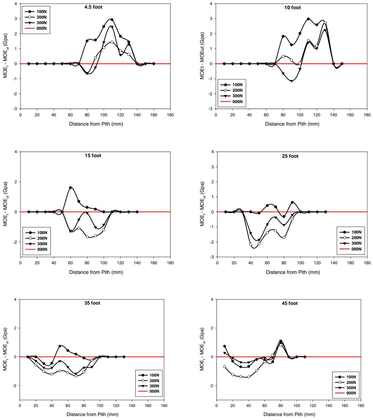
Figure 4.4: Plots of response in modulus of elasticity ( $MOE_t - MOE_{ut}$ ) versus radial distance by treatments at different height levels.
