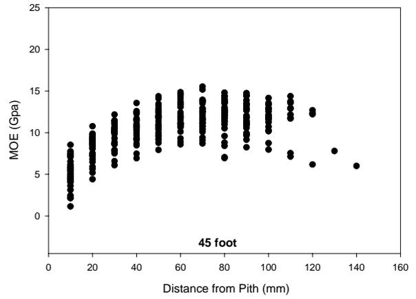
Figure 4.1: Plots of modulus of elasticity (MOE) versus radial distance at different height levels.
