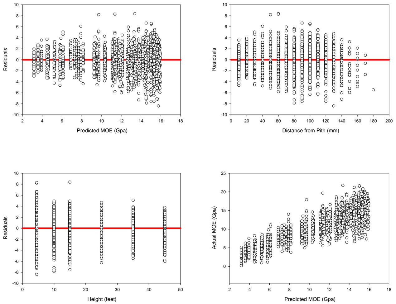
Figure 4.5: Residual plots versus independent variables and actual modulus of elasticity (MOE) values versus predicted values for nonlinear MOE model.
