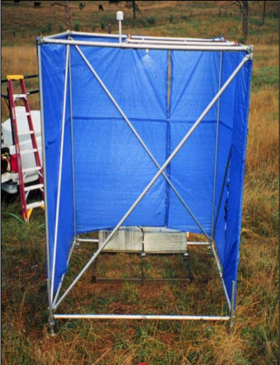
Figure 6. JOERNS INC. rainfall simulator fitted with tarps to provide a windscreen.
