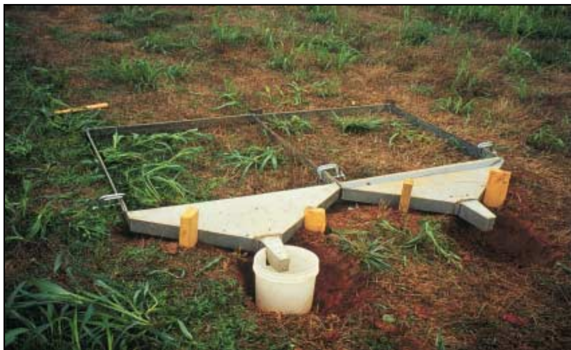
Figure 5. Flumes were installed at the down-gradient edge of each plot to divert surface runoff to a collection point.
