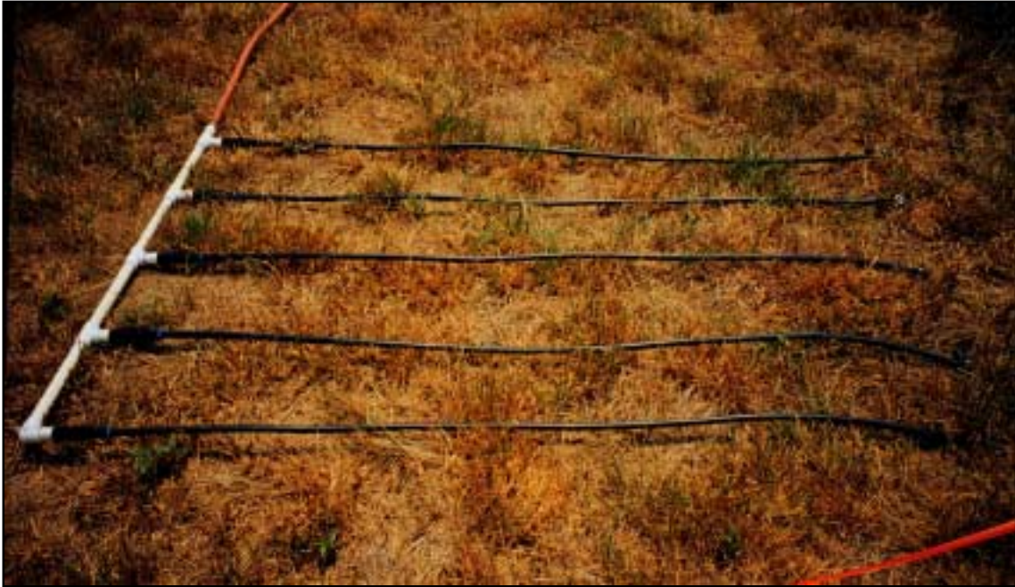
Figure 2. Drip-irrigation system used to pre-soak field plots.
