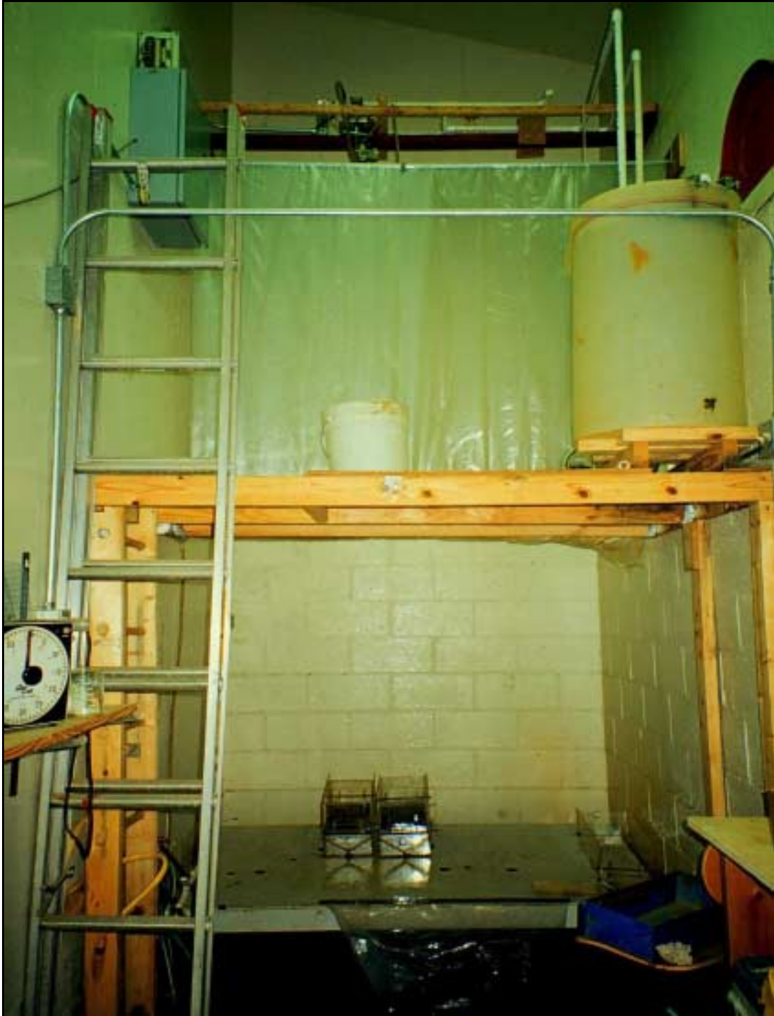
Figure 8. Indoor rainfall simulator.
