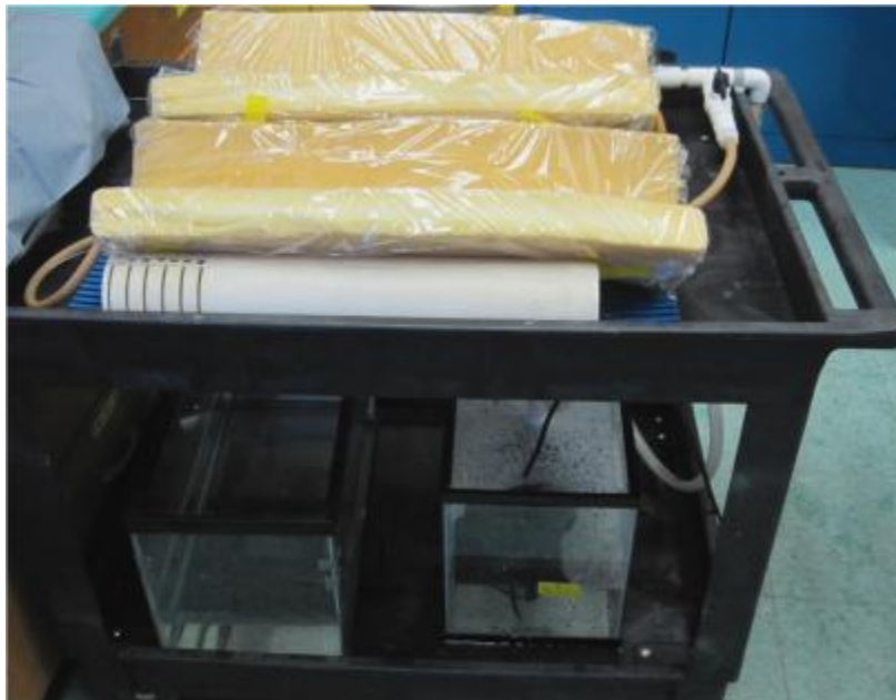
Figure 3.2 The re-circulating anesthesia delivery system used during surgery for the evaluation of physiological and pathological effects of intracoelomic transmitters in Siberian sturgeon. Data was collected in January 2010.
