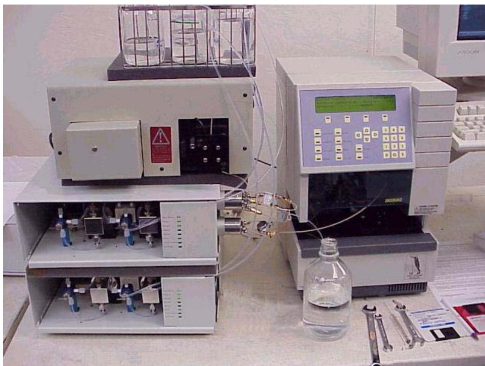
Figure 2.1 A photograph of a Micro-Tech Ultra Plus II MD capillary HPLC system. The image was extracted from http://www.microlc.com/newweb/2Dsetup12.htm .
