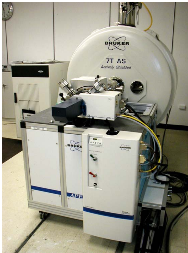
Figure 2.6 A photograph of a FTMS-130 intermediate pressure MALDI source coupled to a 7.0 tesla Bruker BioApex Fourier transform mass spectrometer.
