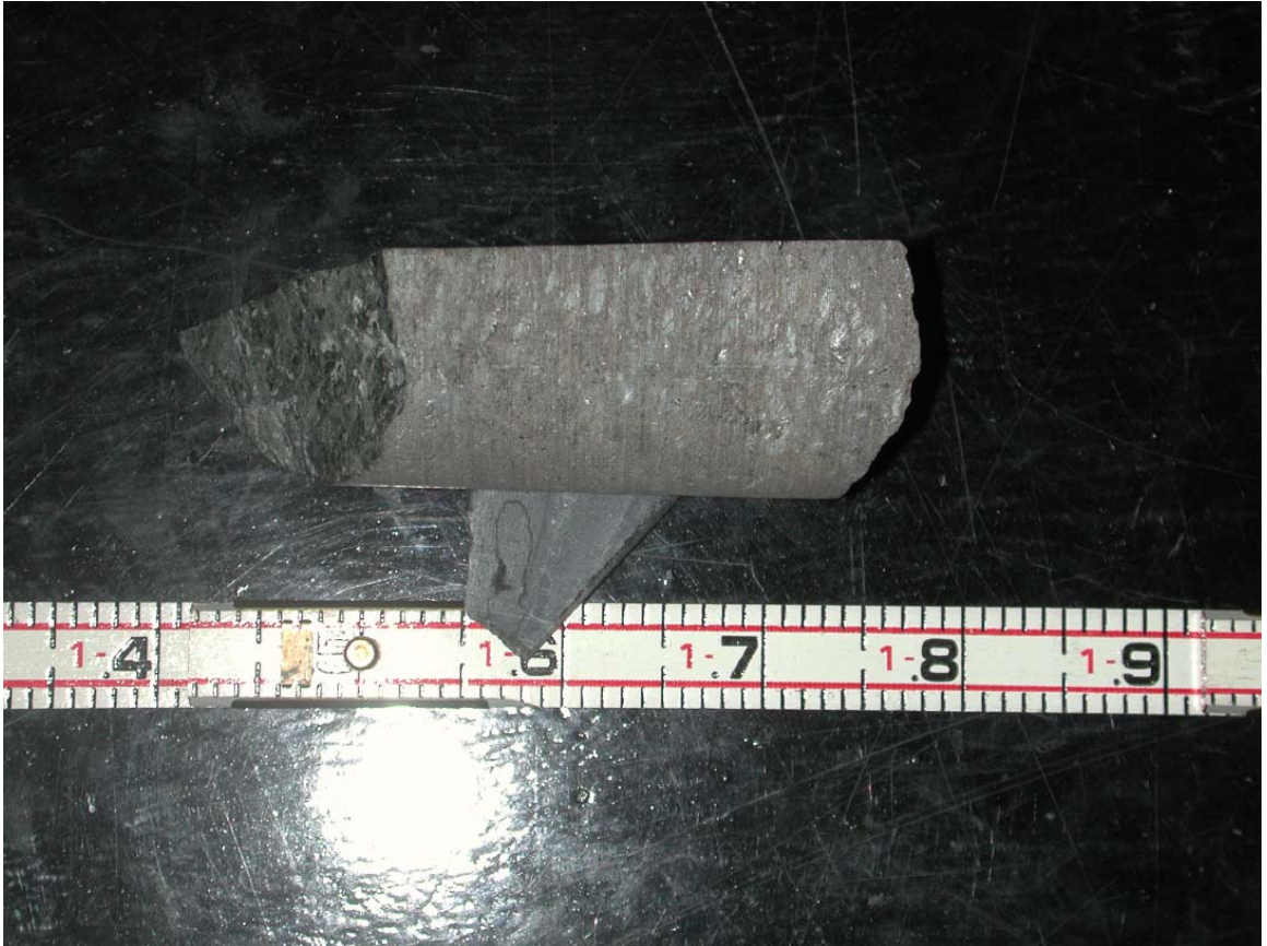
Figure 2.1. Representative drill core cut in half; perpendicular to foliation.
