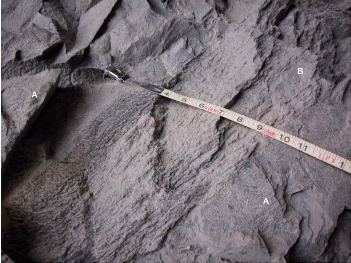
Figure 3.1. Interlayering between quartz mica schist (A) and mica schist (B). Taken from Chattahoochee Tunnel, south end, 53 m below ground surface (bgs).
