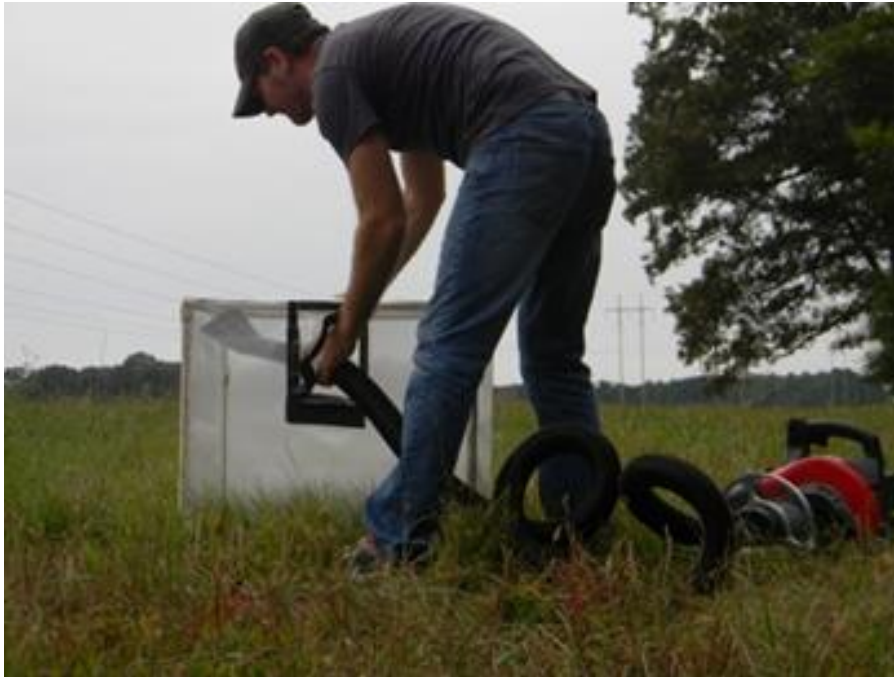
Figure 2.1. Cage constructed of a pvc frame, mesh fabric fixed to 4 sides, with open bottom and clear acrylic sheeting on top. If flies were too numerous to be counted they were captured with vacuum.
