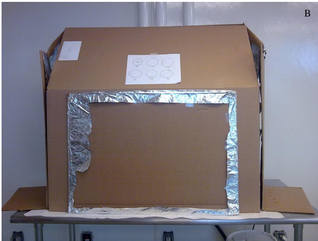
Figure A.1. UV lamp apparatus without the front cardboard shield (A). UV lamp apparatus covered with cardboard lined with aluminum foil during UV exposure (B).
