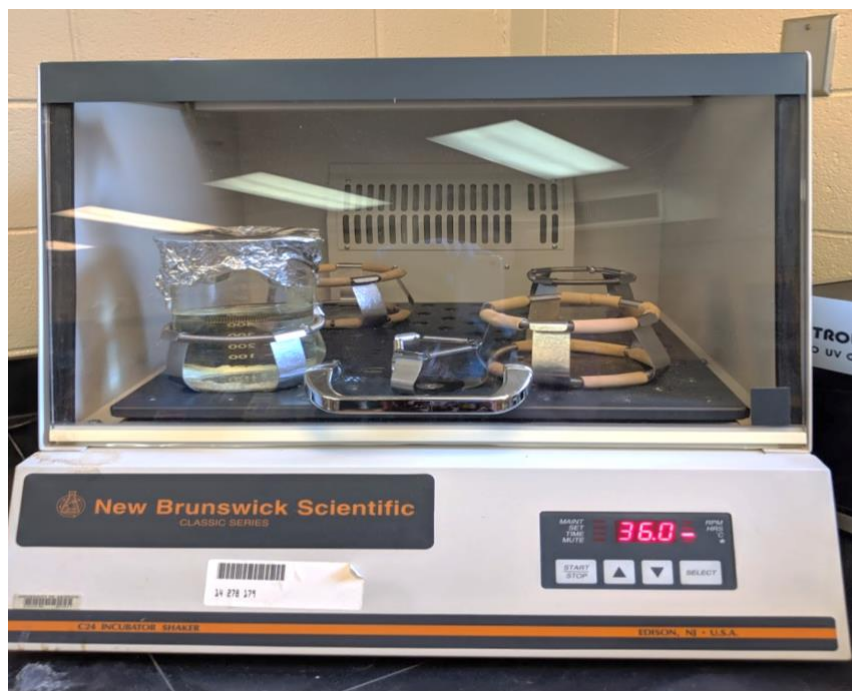
Figure 4.1: Kinetic release study of microparticles suspended in ethanol (using New Brunswick C24 incubator shaker at 100 rpm and 37 \pm 2 °C)
