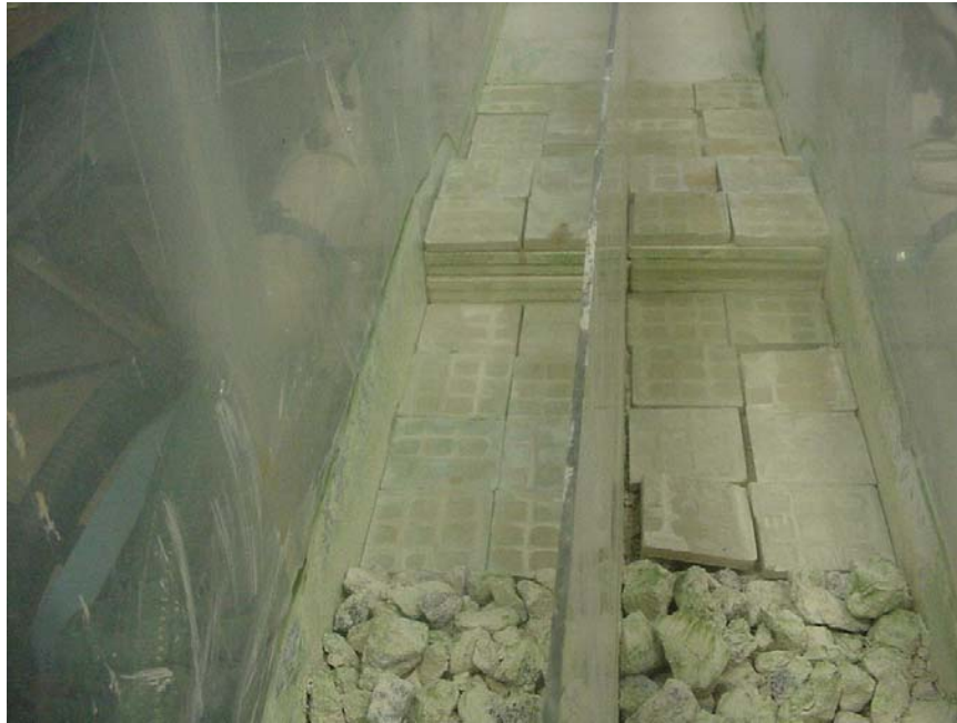
Figure 2.1 Laboratory flume setup showing the rock bottom and tiled zone up-stream from the weir and the tiled zone below the weir.
