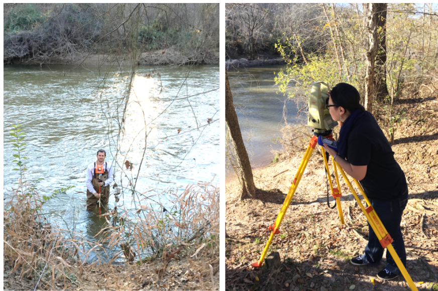
Figure 4.4: Bathymetry data collection on the Middle Oconee River near Athens, Georgia.
