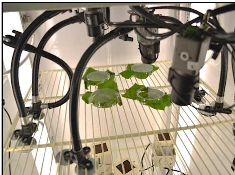
Fig. 2.2. Treated leaf bioassay with experimental arenas positioned below digital video cameras.
