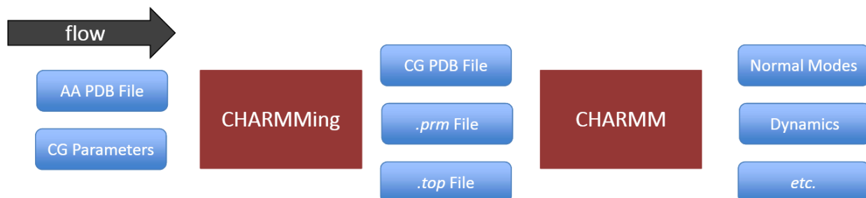
Figure 5.1 A flowchart demonstrating how the CG model builder in CHARMMing interacts with the underlying CHARMM functionality.
