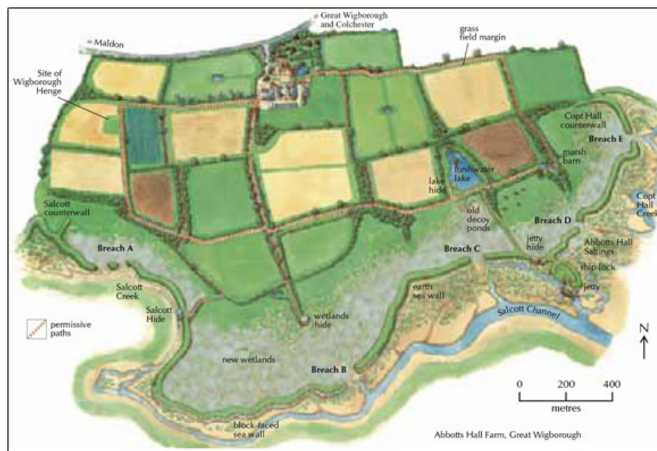
Figure 5: Schematic plan of managed realignment in Abbots Hall Farm, Essex, UK (UK EA, 2010).
