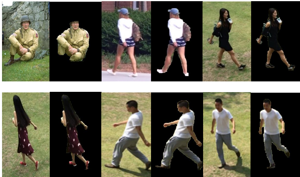
Figure 17 Results of automatic GrabCut. The pedestrians are extracted from the background and only a very small part of the background left.
