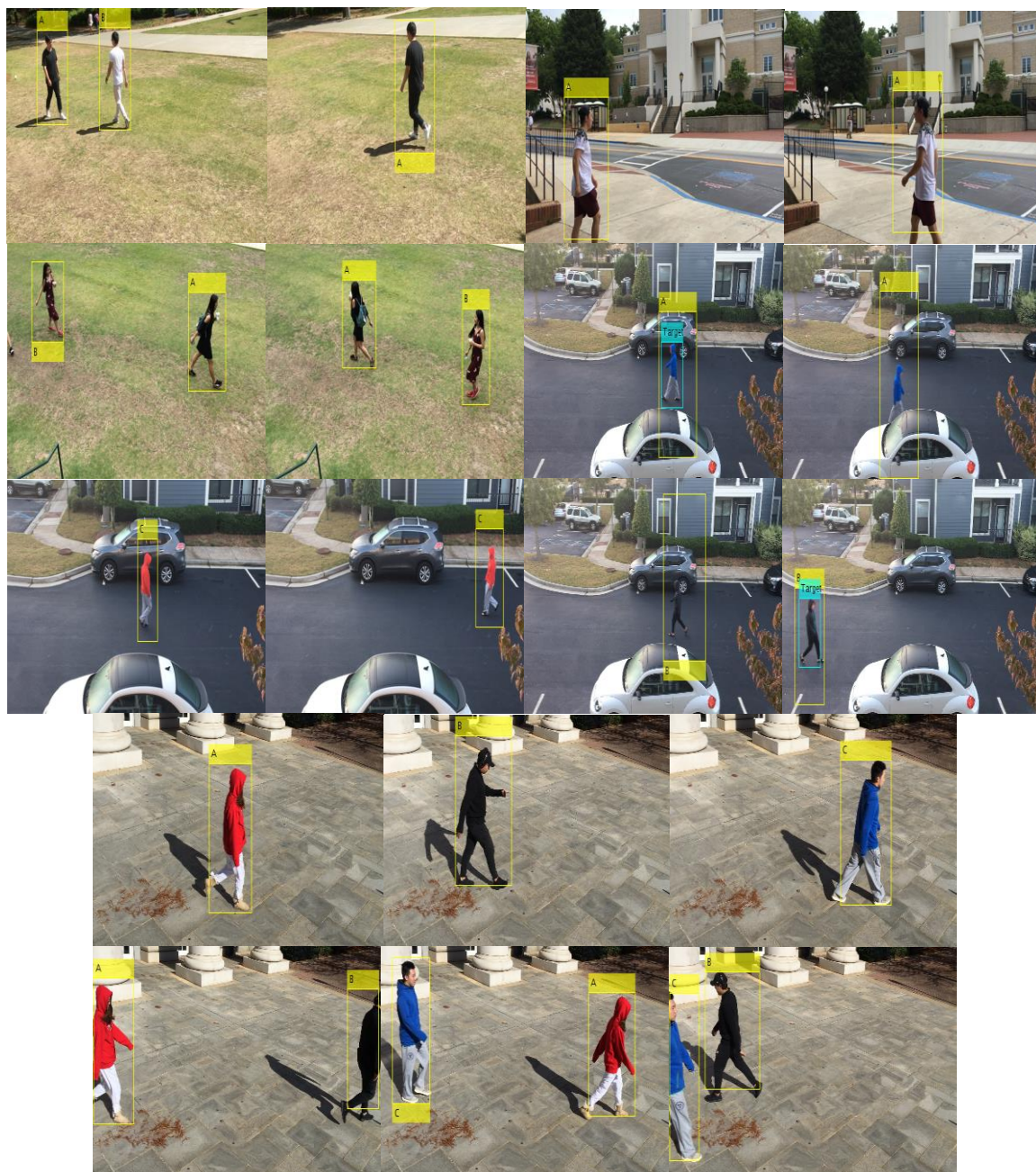
Figure 20 Results of re-identification. Same pedestrians are labeled with their original label when they come back into the video again.
