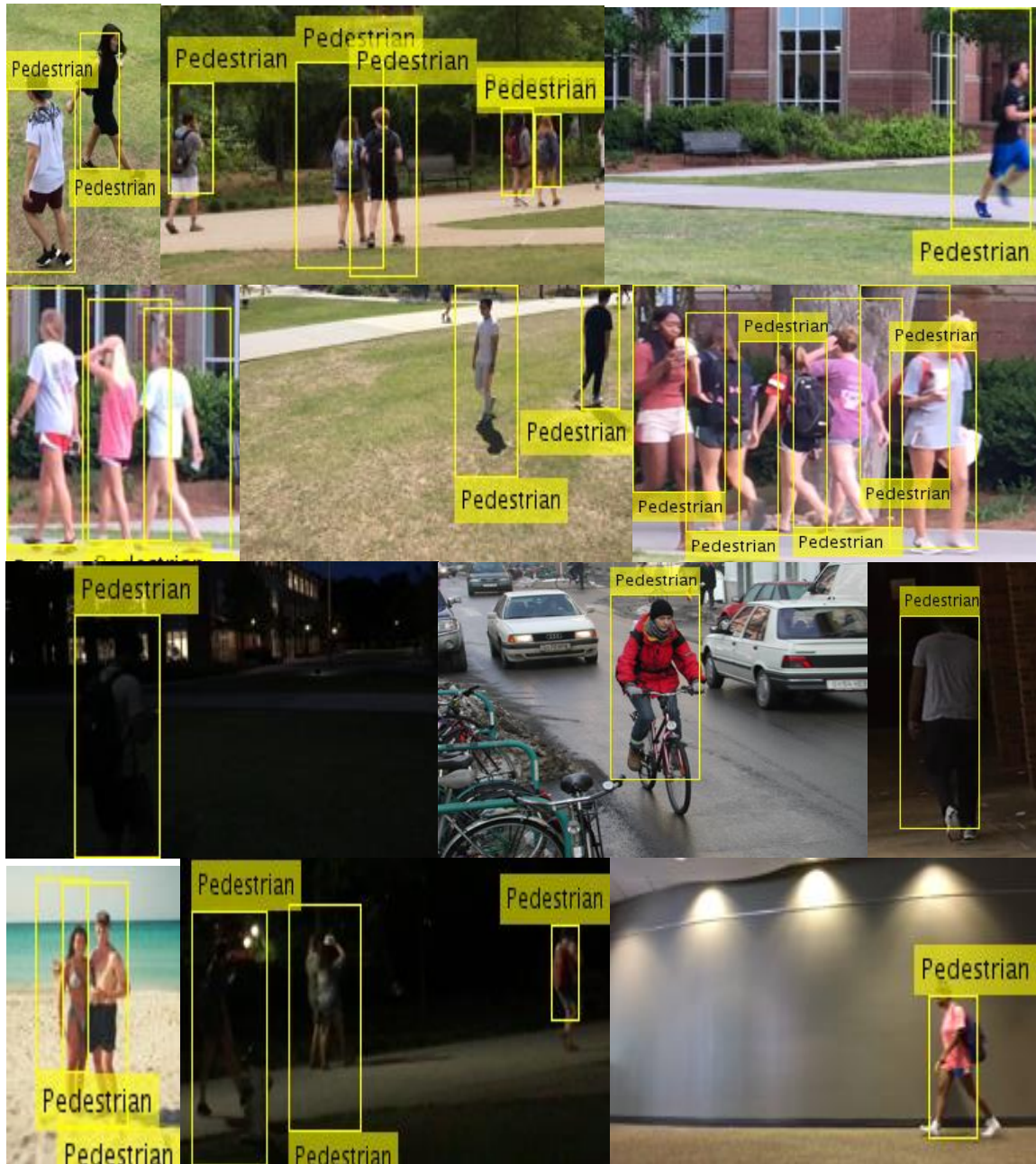
Figure 15 Successful results for pedestrian detection using the neural network. All the people in those images are marked by a yellow rectangle and labeled as a pedestrian.
