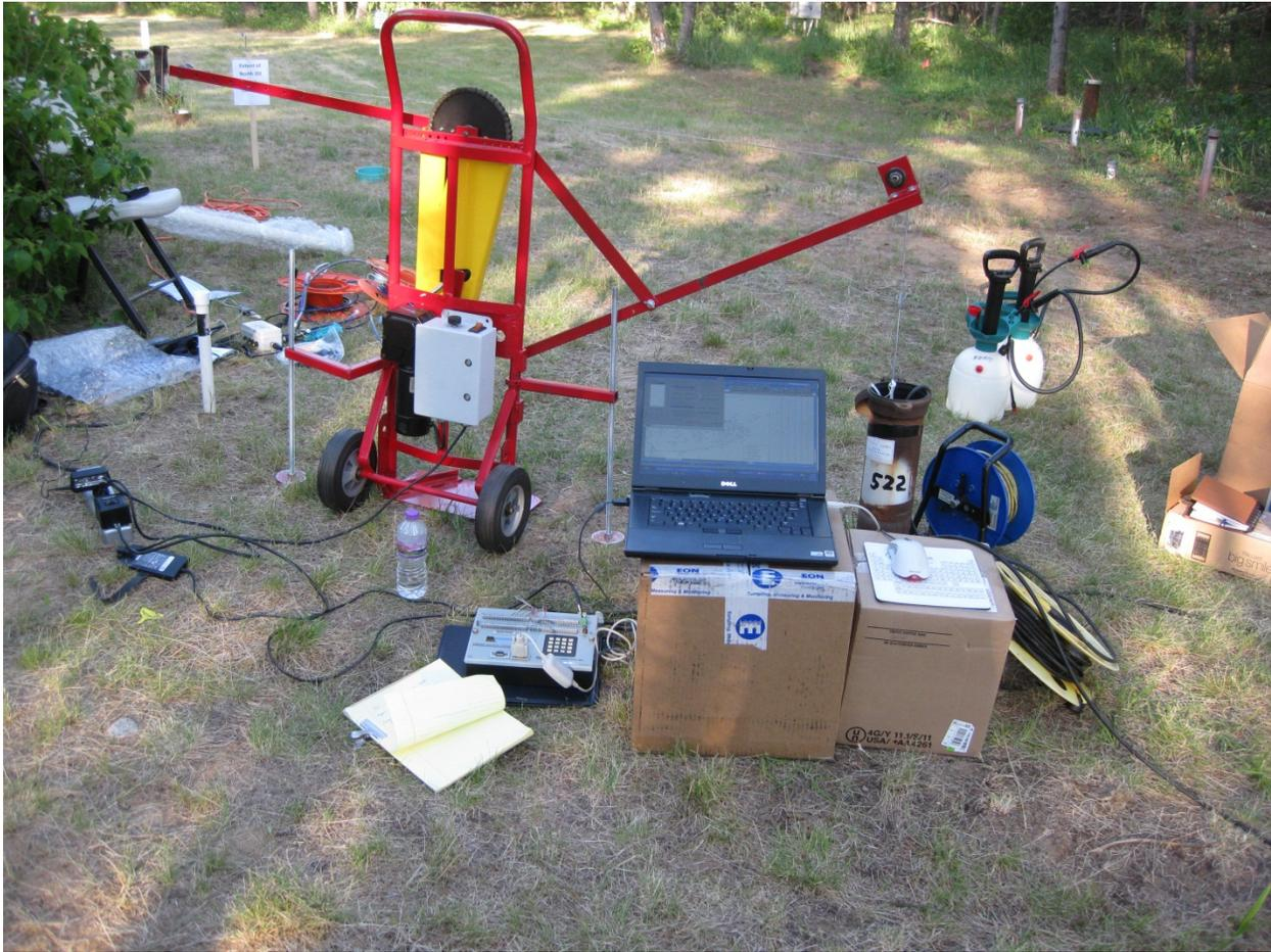
Figure 4.2. Photograph of the oscillating slug test device set up to begin a test at a site control well.
