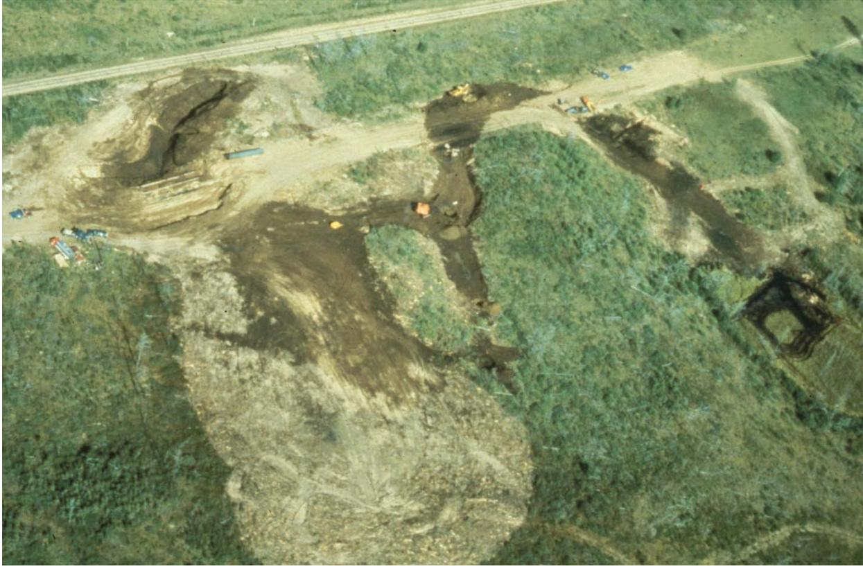
Figure 3.1 Oblique aerial photograph looking east of the August 1979 crude oil release site, including an open recovery trench in the North Pool area (upper left), and surface staining along the sinuous flowpath of oil to a wetland located approximately 200 m south of the release point (lower right; Delin, 2012, personal communication).
