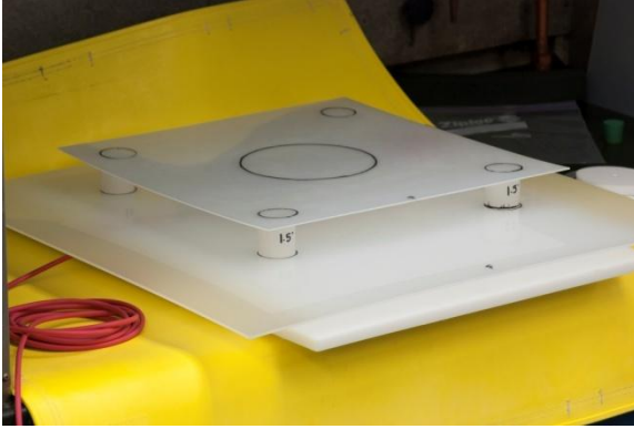
Figure 3.2: Outlines on dielectric barriers used to accomplish parallel placement of electrodes.
