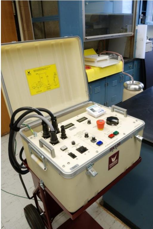
Figure 3.1: Entire plasma generation system with control box, high-voltage transformer, electrodes, and dielectric barriers.
