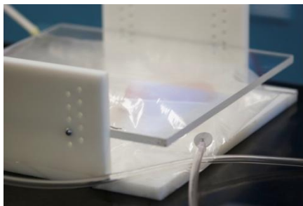
Figure 3.4: Filling station with inlet MA gas and outlet vacuum for flushing sample.
