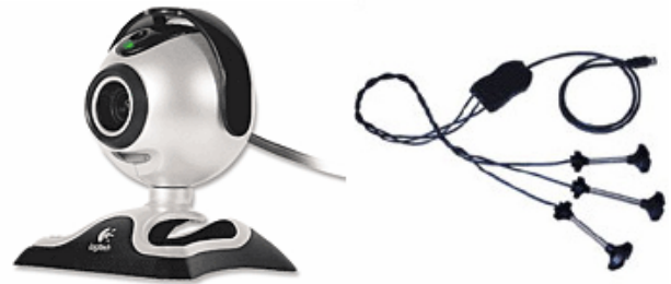
Logitech QuickCam Pro 400 (Left) evolution robotics IR sensor pack (Right)
