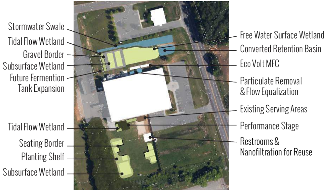
Figure 58. Proposed Site Plan for Wastewater Treatment at Terrapin Beer Co. (diagram by author)
