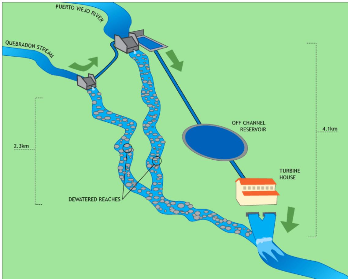
Figure 3.3. Schematic showing the operations of most hydropower projects in Sarapiquí. The dam(s) blocks flow and diverts water into a tunnel or pipeline to a reservoir. Water is run down a gradient to turbines and used to generate electricity and then returned to the river. This figure is based on the Doña Julia Hydroelectric Center, which operates with dams on two rivers. (Figure courtesy of Chesley Lowe).
