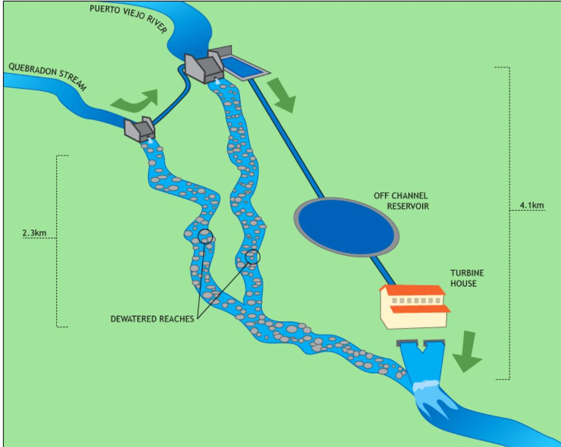
Figure 5.9. Example of diversion dam operations. Water is diverted from the river into a tunnel or pipeline. River water is stored in an off-channel reservoir until peak hours of demand, then run down a gradient to a turbine house. Water is used to generate electricity and then returned to the river. This schematic is based on the Doña Julia Hydroelectric Center that operates on the Puerto Viejo River and the Quebradon stream. (Figure by C. Lowe)
