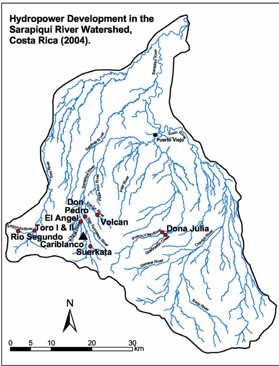
Figure 3.2. Hydropower development in Sarapiquí is concentrated in the upper watershed where there are abrupt changes in elevation. The locations of eight existing hydropower projects are indicated by a red circle on the map. The site for the proposed Cariblanco hydropower project is indicated with a black triangle. Also, the old gauge on the Sarapiquí River is just downstream from the town of Puerto Viejo, before the confluence of the Sucio River. (Figure by M. Snyder).
