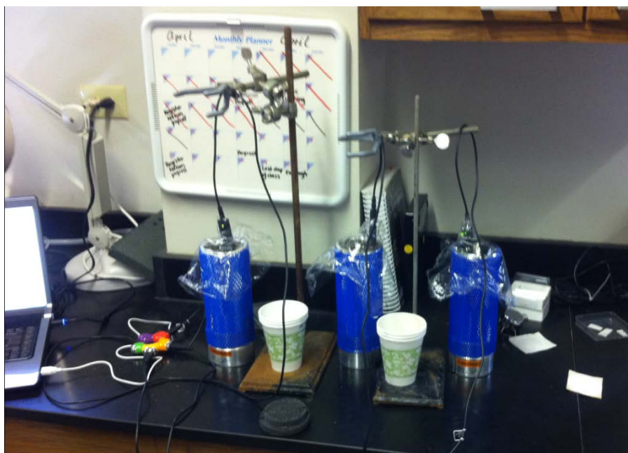
Figure 3.7: The experimental set-up for the calorimeter study.
