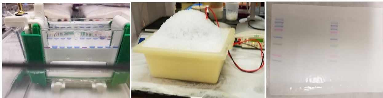
Image 2: Electrophoresis chamber with loaded SDS-Page gels. The ladder is the darker purple in the 1 st and 4 th positions on the gel. The volumes loaded into the lanes contain 30 \mu\text{g} of protein per sample.
