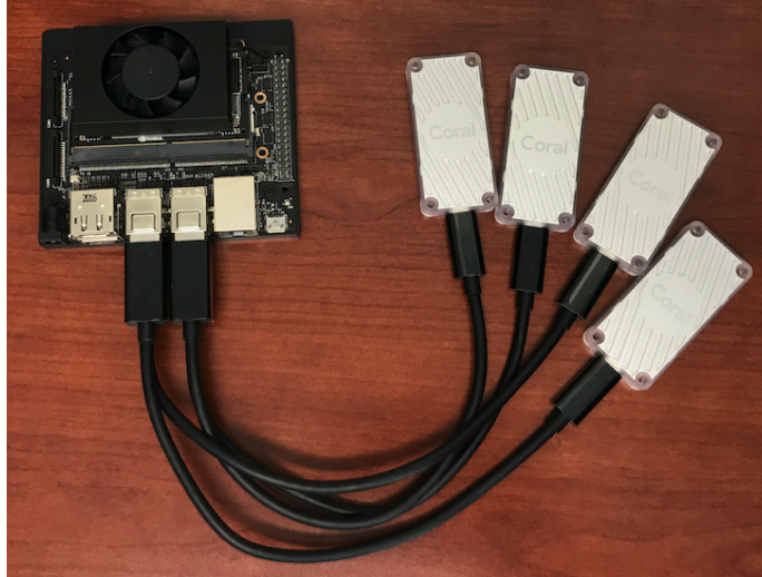
Figure 4.15: EdgeTPU-cluster composed of four EdgeTPUs (USB-Accelerator) connected with J.Xavier
