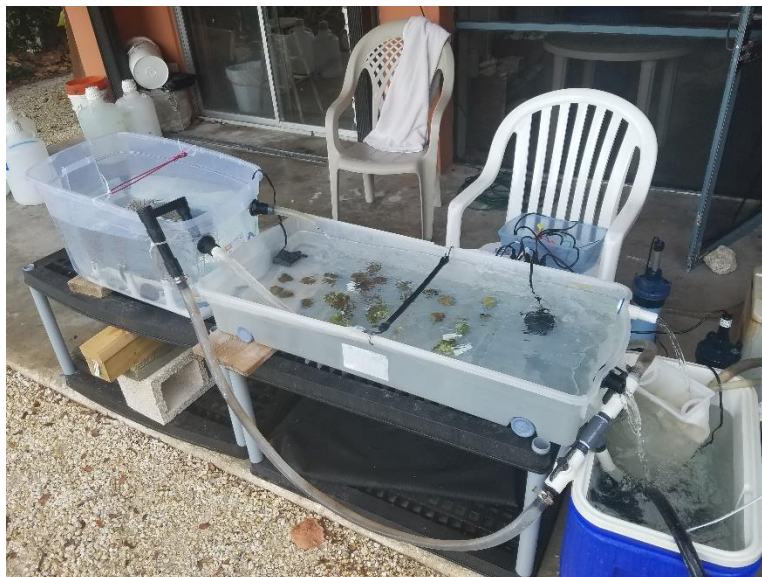
Figure 2. Specimen holding tanks. Antilloorgia , Gorgonia ventalina , Plexaurella , Acropora palmata , were suspended in the larger tank on the left to reduce stress. Macroalgae and smaller hard coral chunks were kept in the tank on the right. The filtering system can be seen to the right side of the image.
