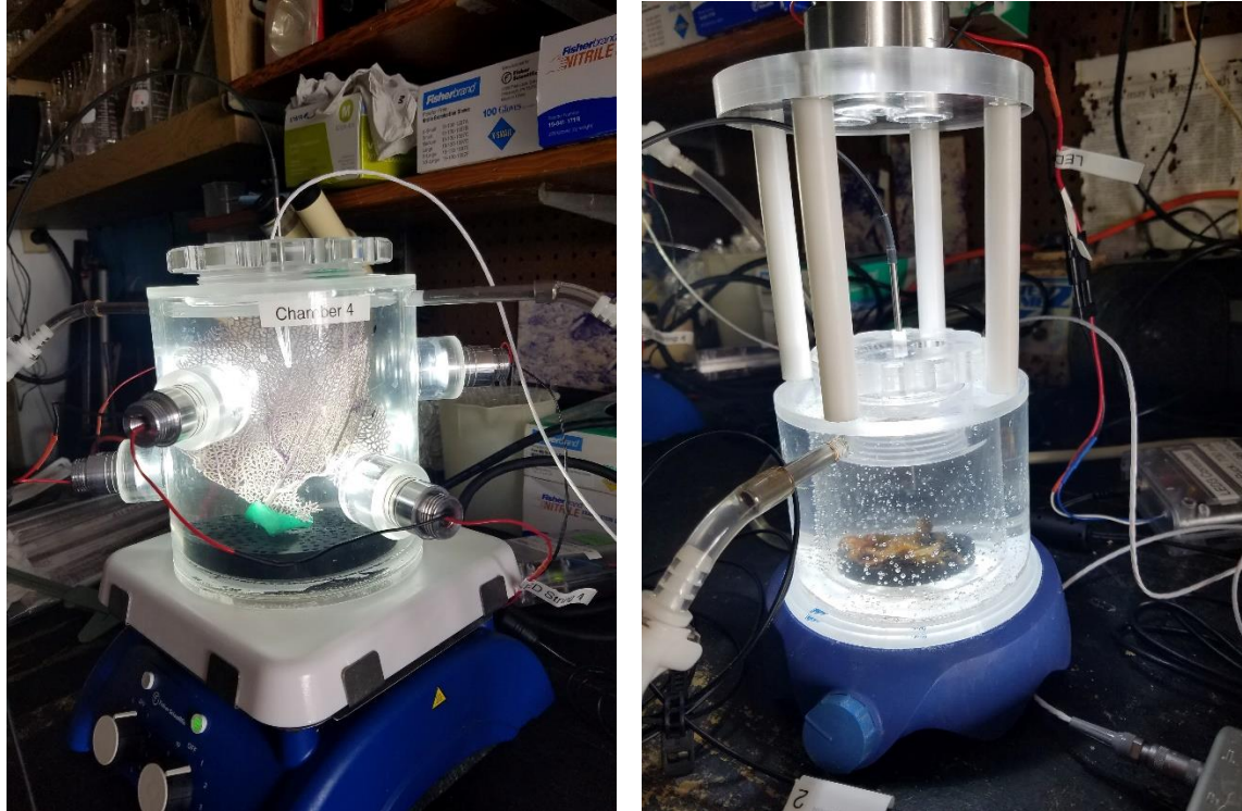
Figure 3. Chambers and light set ups used for metabolic measurements. Left picture is the 1200 mL chamber used for larger specimens, light shines on these specimens from the side. Right picture is the 140 mL chamber used for smaller, flatter specimens. Light shines on these specimens from above.
