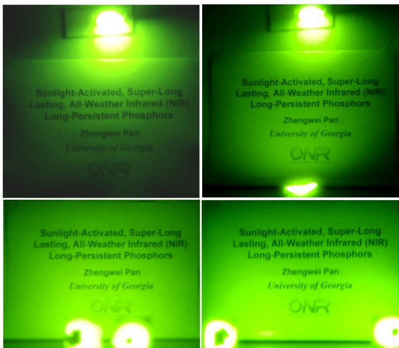
Figure 4.18 NIR afterglow photos of sunlight-activated \text{Zn}_3\text{Ga}_2\text{Ge}_4\text{O}_{14}: 0.1\%\text{Cr}^{3+} disks used as efficient, secret lighting sources in the dark. The photos were taken by a digital camera with a night vision monocular.
