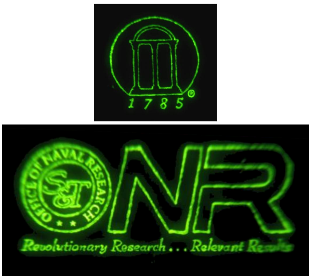
Figure 4.19 NIR afterglow photos of the logos of the University of Georgia (UGA) and the Office of Naval Research (ONR) written with the paint made from \text{Zn}_3\text{Ga}_2\text{Ge}_4\text{O}_{14}:0.1\%\text{Cr}^{3+} phosphor powders with acrylic polyurethane varnish. The photos were taken by a digital camera with a night vision monocular. The quantity of the phosphor powders in the varnish is 30 wt. %. The logos were exposed to sunlight for 5 minutes. The logos can be clearly seen after 100 h with the night vision monocular.
